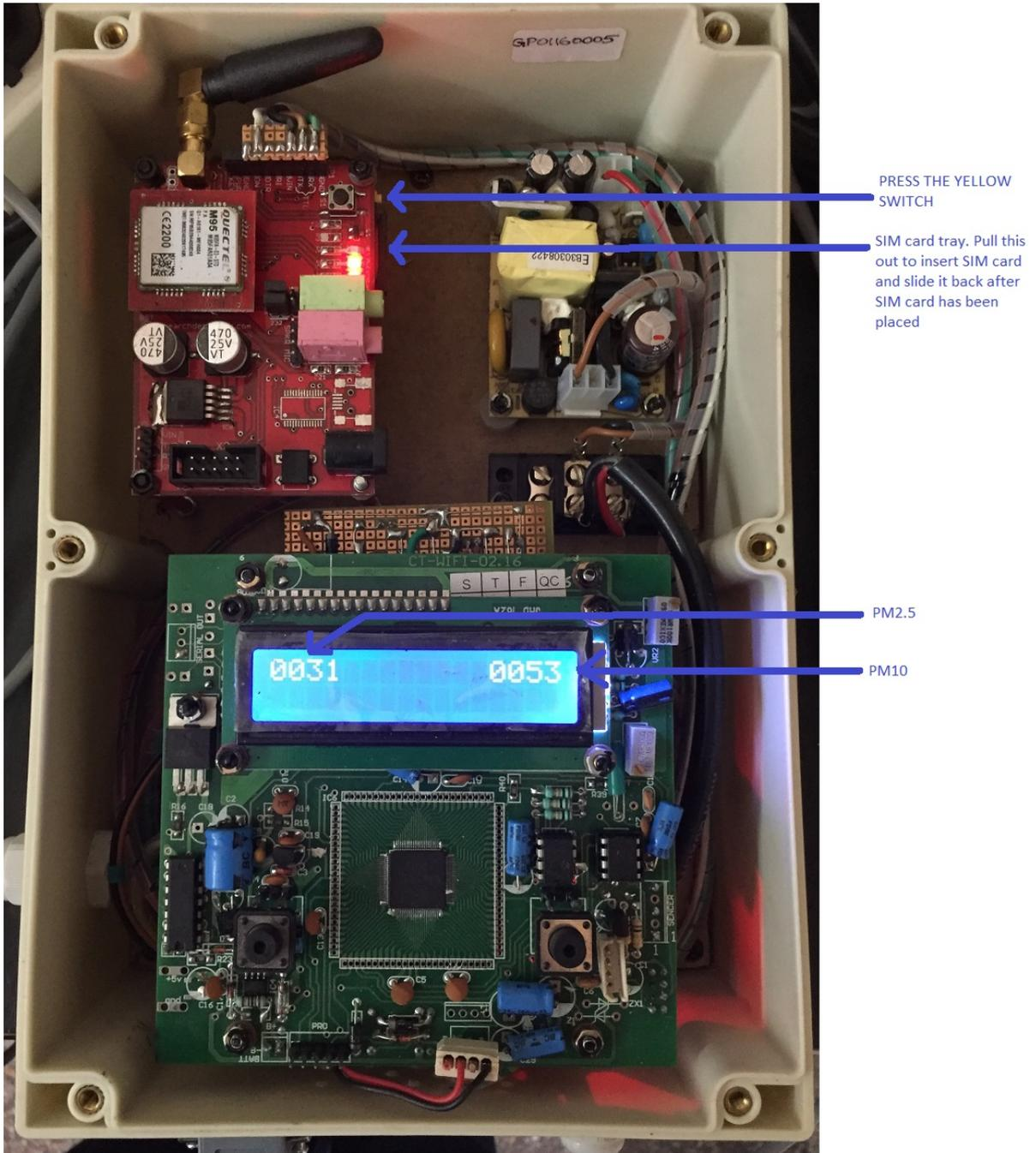
3. Now on the top left side, there is a PCB with an antenna. This is the GSM modem module.
